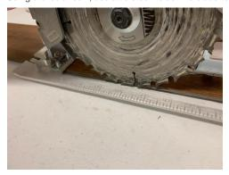
3. Carefully, cut the plank along the mark. Take care not to damage the adjacent plank. CAUTION; wear the appropriate eye protection, respiratory equipment and be certain that the safety guards are in place and operational
